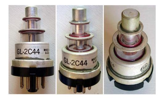
Similar to <u>GL-446</u>, this triode was designed with a larger anode cap, to increase its power handling capability. It can be replaced by <u>2C43</u>.
