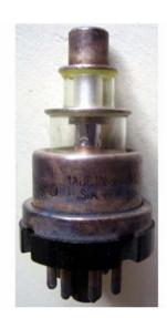
UHF lighthouse planar triode intended for use as class-C amplifier or pulsed oscillator at high frequencies. Probably derived from the <u>2C40</u>, with increased cathode and anode surfaces.
