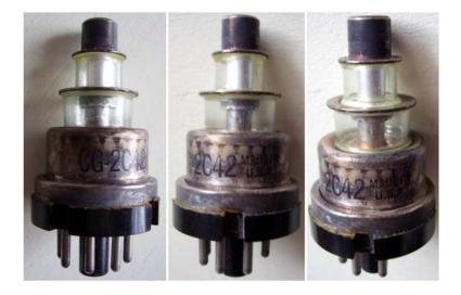
UHF lighthouse planar triode intended for plate pulsed operation.
