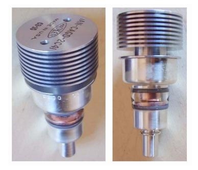
"Oil-can" shaped planar triode, 2C41 is a variant of 2C39 for pulse operation, same format but not physically interchangeable. Non registered code of the GE ZP602 design.
