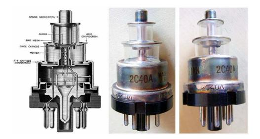
Lighthouse planar triode. One of the early planar triodes developed during WWII, 2C40 replaced the very early lighthouse type <u>446A</u> designed by General Electric.
