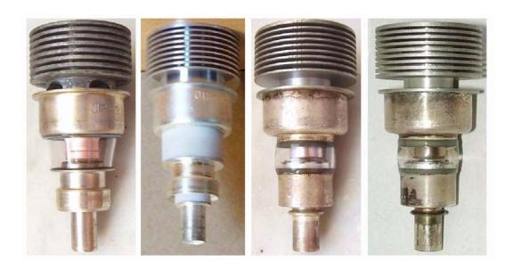
'Oil-can' shape UHF planar triode. The large finned plate radiator grants up to 100W dissipation with forced ventilation. General Electric design, 2C39 derives from the GE experimental tube known as <u>L-14</u>. Introduced during WWII, it was registered only in 1946. Special selection 2C39 with relaxed specs was offered as 2C38.
