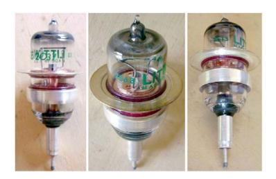
UHF planar triode, 'rocket' style. Was introduced by Sylvania as SB846A during WWII. Also manufactured by Litton.
