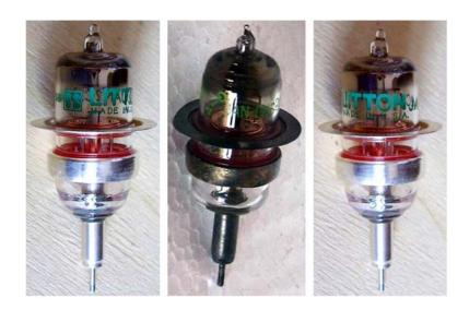
2C36 was one of the most popular 'rocket' style planar triodes, registered to Sylvania for operation even beyond the upper limit of UHF, 3 GHz and over.
