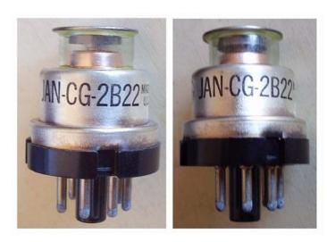
Planar 'lighthouse' diode proposed as TR switch, UHF mixer or detector.
