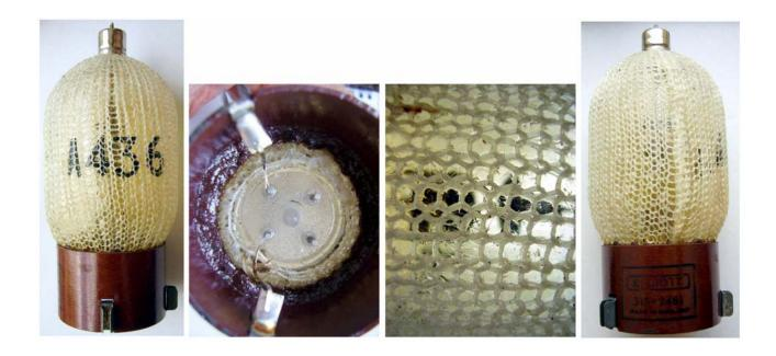
Three electrode spark gap 'Trigatron' for delay line discharge/pulse forming in radar modulator circuits.
