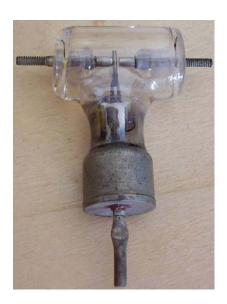
SPDT mechanically-actuated vacuum switch, designed for radio-frequency operations.
