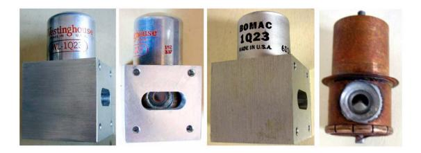
X-Band vacuum reference cavity, waveguide mounted. 9280 MHz resonant frequency. Q unloaded from 1900 to 2400.
