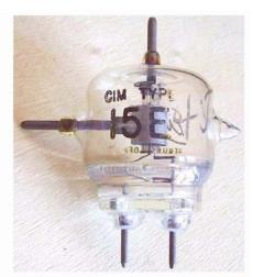
This small power triode was also known as 4C30, 8023 or 3-15A3. Capable of 20W anode dissipation, 15E could be used up to 500MHz.
