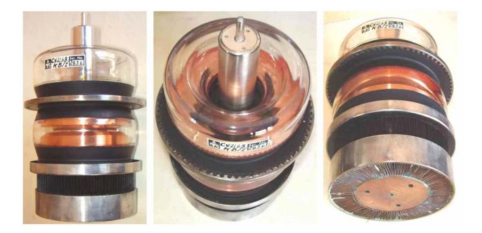
Forced-air cooled transmitting triode. 1500 W anode dissipation. 1.5 kV anode voltage at 1700 mA cathode current. Up to 11 kV in pulsed operation. Usable with external coaxial cavity up to 600 MHz.
