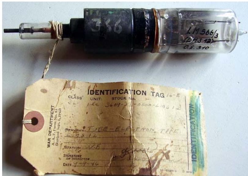
Fig. 1 - This sample of LMS 12 looks unused. On the glass bulb an alternate marking as LM 566/3 is well visible. It still retains its US War Department classification tag, dated 1946. The rod on the left looks to be the center conductor of the coaxial output. The two heater/cathode pins are on the right of the large glass bulb. Click on the image for more details.
