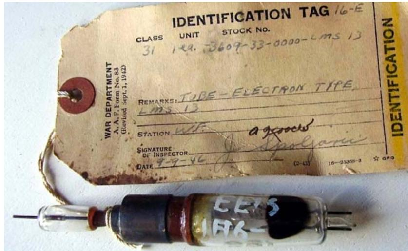
Fig. 2 - LMS 13 sample in like-new condition, still retaining its US War Department classification tag, dated 1946. 1.625 cm, 5 kW. 18-resonator anode system. Click on image for full available information.
