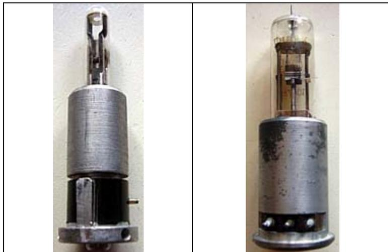
**Fig. 4 - Left, the RD2Mh could deliver 300 mW CW from 4.3 to 5.5 GHz. It was capacitively coupled to the external resonator. A similar device the RD2Md was used as local oscillator, as off-the-shelf replacement for the British klystron, in the receiver of the Berlin microwave set. Right, MD4Ma was designed to operate from 1.1 to 1.6 GHz, delivering about 15 W CW. Click on each image to access available data.**
