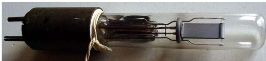
Fig. 3 - Siemens RM4025 looks to be a split-anode, self-contained resonating system magnetron. It was designed for operation at 3 cm. Still in evaluation phase at the end of the war. The sample still retains its US War Dept. classification tag, dated 1946. Click on image for full available information.
