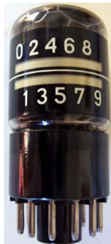
Fig. 9.4 - A sample of Philips EIT beam switching counter with electrostatic deflection. The beam could jump sequentially on a zigzagging trajectory, lighting a dot in correspondence of the reached count.
