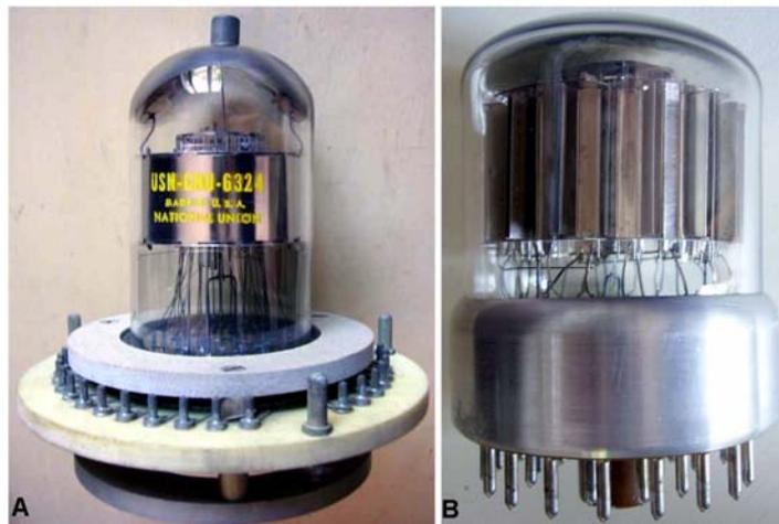
Fig. 9.1 – A) National Union [6324](#) was a beam switched 25-line multiplexer, with 25 control grids, as signal inputs, and a single anode from the top cap. It had to be operated inside a coil assembly which generated a step-by-step rotating magnetic field. B) [6090](#) was a 18-line decoder/demultiplexer, with a single control grid and 18 output anodes all around. (Click the image to enlarge)
