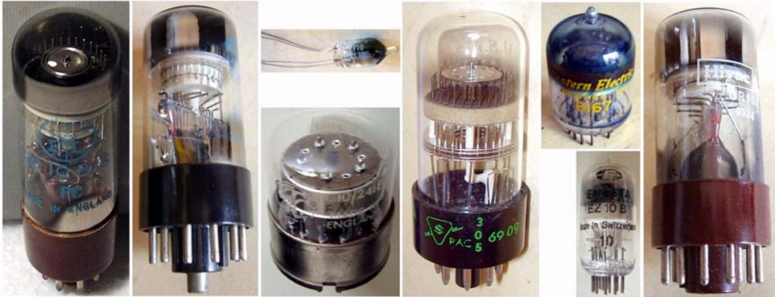
Fig. 9.5 – Samples of gas-filled counter tubes from various manufacturers. The small tube with flying wires in the middle is a gas trigger triode, used to drive counter electrodes.
