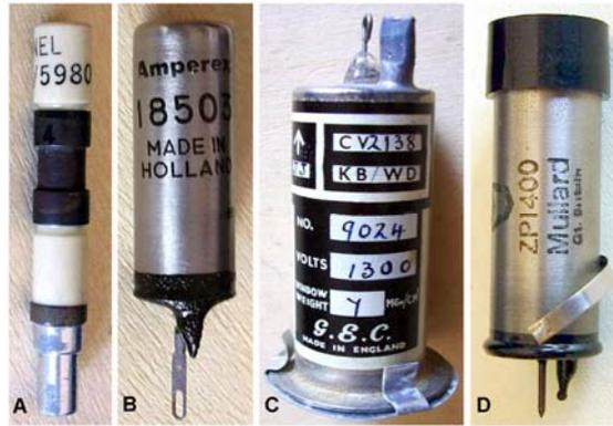
Fig. 8.2.4 - Geiger counter tubes. A) A Lionel [5980](#) cartridge sensor. B) Actually this Amperex badged [18503](#) was made by Philips. D) A British GEC [CV2138](#) Geiger counter. D) [ZP1400](#) was another beta and gamma radiation counter by Philips and related companies.
