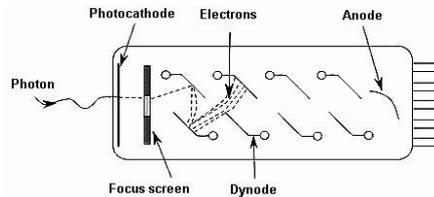
Fig. 8.2.7 - Internal structure of a photomultiplier. Electrons emitted by the photocathode are attracted by the upper first dynode, By secondary emission electrons are multiplied at each impact on a dynode, so that plenty of electrons reach the anode after the travel through eight, or more, cascaded dynode stages.
