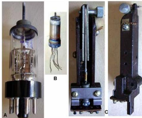
Fig. 8.2.1 - Mechanical displacement sensors. A) In the Russian [6MX1C](#) the plates of two internal diodes are supported by the rod protruding from the top, through a flexible diaphragm. B) The RCA [5734](#) is a triode in which the plate is the internal extension of the sensing tip. C) Two views of a pick-up using the 5734 as active transducer, bottom in the left image. Not sure what the above pick-up was intended for.
