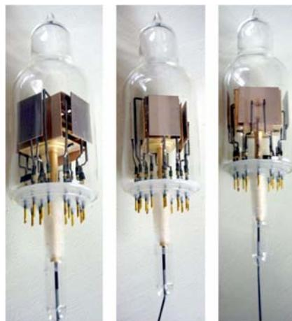
Fig. 8.2.3 - Sample of Philips custom [Omegatron](#). To be cleaned at high-temperature before use, electrodes are made of iridium or osmium. The bulb of this sample is still sealed.
