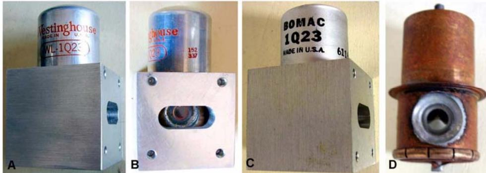
Fig. 7.2.5 - Reference cavities. [1Q23](#) resonates at 9280 MHz with unloaded Q around 2000. Here three photos of cavities complete with waveguide mount and (D) the photo of the copper resonator. (Click on the image to enlarge)
