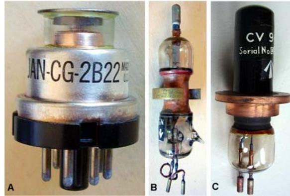
Fig. 7.2.2 - Vacuum diodes used as TR switches. A) [2B22](#) was a General Electric lighthouse UHF diode, also used as TR switch. B) GEC E1248 coaxial diode, approved as [CV8](#), was designed in 1940 to operate as switch in a coaxial line. No known use in operational equipment. C) Marconi DS103, approved as [CV94](#), was used in Type 960 high power radar, switching 450 kW peak pulses at 90 MHz. (Click on the image to enlarge)
