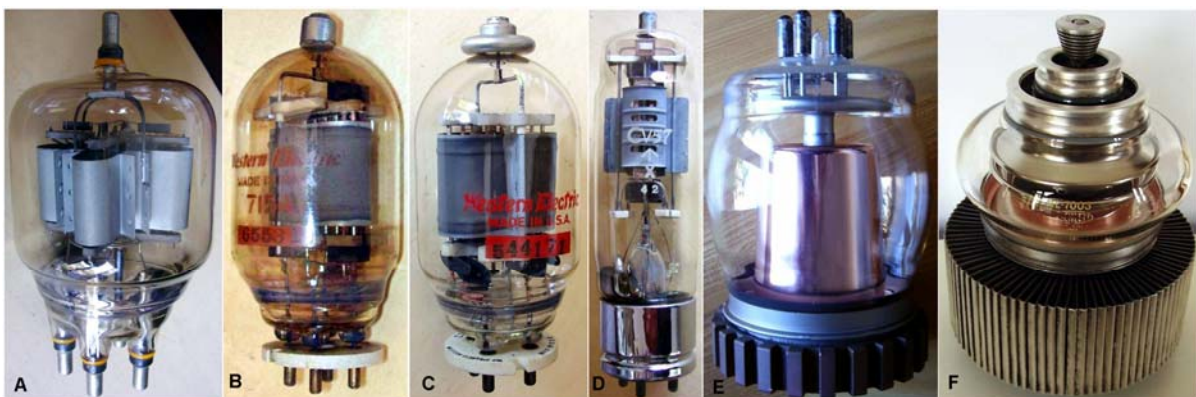
Fig. 7.1.6 - Vacuum tubes designed to operate as power switches in pulse modulators. A) Western Electric 701A was hastily designed to drive the very early WE magnetron, the 700A. The required emission was obtained assembling four electrode sub-systems of the 350A power tetrode, cathode and grids, inside a cruciform plate. Grids were gold plated to decrease secondary emission at high operating temperature. B) 715A was an evolution of 701A for airborne applications. Here the four cathodes were placed side-by-side into a single plate and grid system. 715A evolved through several steps, with improvements of grid cooling and of the insulation. C) 5D21 was a further evolution during the war of 715B, with the addition of a top guard ring to prevent corona discharge at high altitudes. D) CV57 was a quite small British tetrode capable of handling 5 A pulses at 11 kV. E) Amperex AX10318-1 is a tetrode intended to operate immersed in oil to switch 5 A at 100 kV. F) ML-7003 was a screened grid triode used in pulse modulators up to 2.5 MW. It was rated for operation as switch at 40 kV, 80 A.
