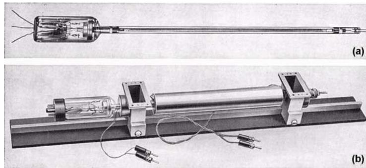
**Fig 6.4.3 – Early TWT prototypes at Bell Telephone. The lower tube is mounted into the waveguide input and output transitions, with the focusing coil between them.**
