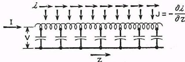
Fig. 6.4.2 – TWT model proposed by Pierce. The helix is here represented as a lumped-constants line and the signal moves forward in the direction  $z$ ; successive arrows, indicated as  $i$ , represent the convection current of the electron beam. The current ( $J$ ) impressed from electrons to the propagating signal is given by the relation on the right.
