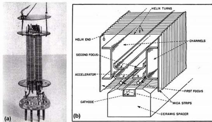
**Fig. 6.4.4 – In the miniature TWT signal enters from the base, travels through the helix and is available on the top. Right, a cross-section view of electrodes. The tube operated in a magnetic field. Electronics, October 1951.**
