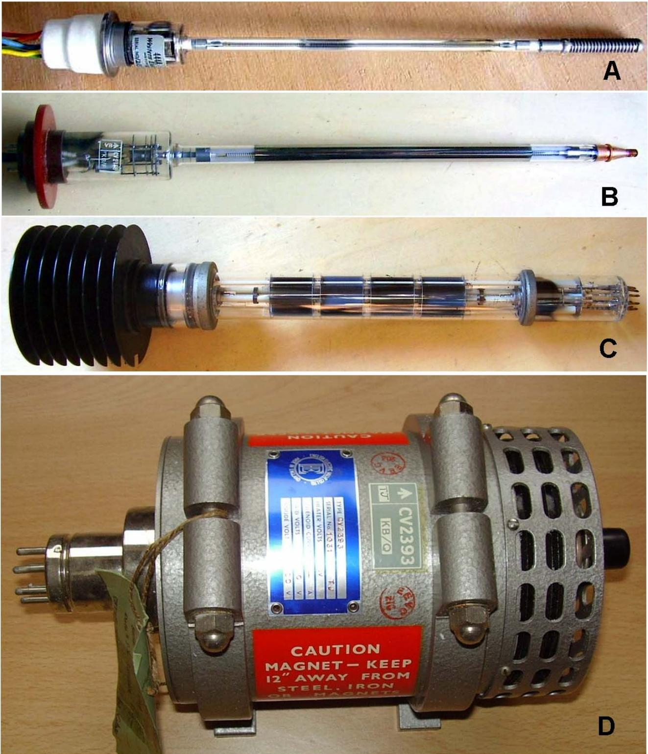
Fig. 6.4.6 - A) Western Electric [444A](#) was one of the early TWTs in volume production for microwave radio relay transmitters. B) British STC [W7/2D](#) (CV2188), introduced in 1957, was tunable from 3600 to 4200 MHz. C) Philips [55340](#) gave in output 8 W typical from 3.8 to 4.2 GHz with 50 mA beam current. D) [CV2393](#) was a backward-wave oscillator (BWO) used in electronic countermeasures, tunable from 7 to 11.5 GHz.
