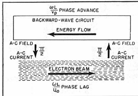
**Fig. 6.4.5** – The RF field is propagated in the transmission line from right to left, with a phase velocity slightly lower than the velocity of the electron beam, which moves from left to right. On the left energy is transferred from the line to the beam, on the right it returns back to the line, each transfer adding 90-degree phase lag.
