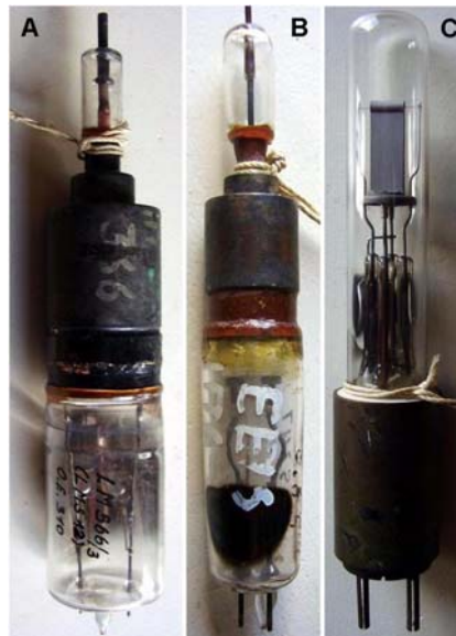
Fig. 6.3.4 - Three German magnetrons in excellent conditions are the rarest of the whole collection. A) One extremely rare sample of the X-band 12-cavity LMS 12 , used in the very late Berlin D radar sets. Only few tens of units made before the end of war. D) The 18 GHz version LMS 13 remained in the evaluation stage. This is the only sample still intact to survive. E) Even more rare this RM 4025 , a split-anode self-contained-resonator pulse magnetron in a developmental stage at Siemens. 5 kW pulses at 10 GHz. (Click to enlarge)
