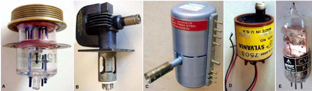
Fig. 6.3.8 - Small postwar magnetrons. A) This interdigital Sylvania experimental 3J22 could operate at 25.000 pps with 4 \mu s pulse duration. B) 5609 was a 70 W continuous wave type intended for RF heating. C) 6177A was a vibrating-reed FM modulated magnetron designed for radio-altimeters. D) 7503 was a tiny X-band magnetron, 200 W output pulses, for beacon applications. E) British CV2380 was an external-cavity X-band magnetron for beacons. It operated in a spatial-harmonic mode. (Click on image to enlarge)
