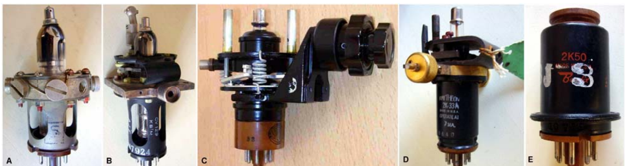
Fig. 6.2.4 - More klystron tubes developed during WWII. A) CV238 , capable of operating at 250 volts, was introduced in 1943 to replace high voltage types, as CV35, in airborne applications. B) CV129 , a British X-band klystron, was readily phased-out in favor of 723A/B. C) 2K41 was one of the many klystron devices designed by Sperry during the war. D) 2K33A , the first K-band klystron, was the result of a design performed in England at Clarendon and perfected in America by Raytheon. E) The electronically tuned 2K50 was the refined WE answer to 2K33. (Click on image to enlarge)
