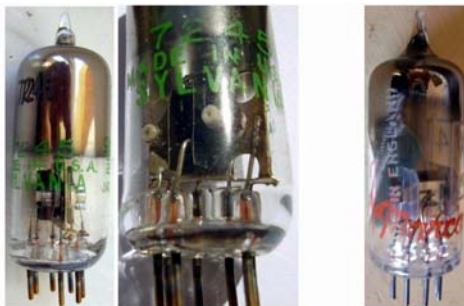
Fig. 5.18 - Left, two views of the Sylvania 7245 , a byproduct of a research contract with Bureau of Ships to build a fully automatic tube production plant which led to the ceramic triode SDN-1724D. Right, the British Marconi A1714, approved as CV408 , capable of operating as low-noise amplifier or oscillator up to 1000 MHz. (Click on the image to enlarge)
