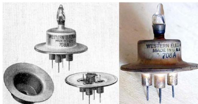
Fig. 5.14 - Left, shape and internal details of the WE 708A grounded-grid triode. Grid was welded to the steel case. Right, a sample of the tube on exhibit at the collection. Tung Sol second sourced this tube. (Click on the image to enlarge)
