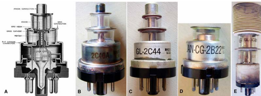
Fig. 5.9 - Lighthouse tubes were designed during WWII by General Electric. A) Construction details of a 2C40, showing the planar electrodes held in place by the two glass spacers. B) 2C40 could be used up to 3.75 GHz. As oscillator in pulsed operation it could deliver 300 W. C) Larger cathode surface and electrodes were used in this 2C44 to generate more powerful pulses, up to 1.4 kW. D) The 2B22 planar diode was intended to operate as detector, mixer or TR switch up to 1.5 GHz. E) 3C22 was the most powerful device in the family, capable of dissipating 125 W with forced-air cooling. (Click on the image to enlarge)
