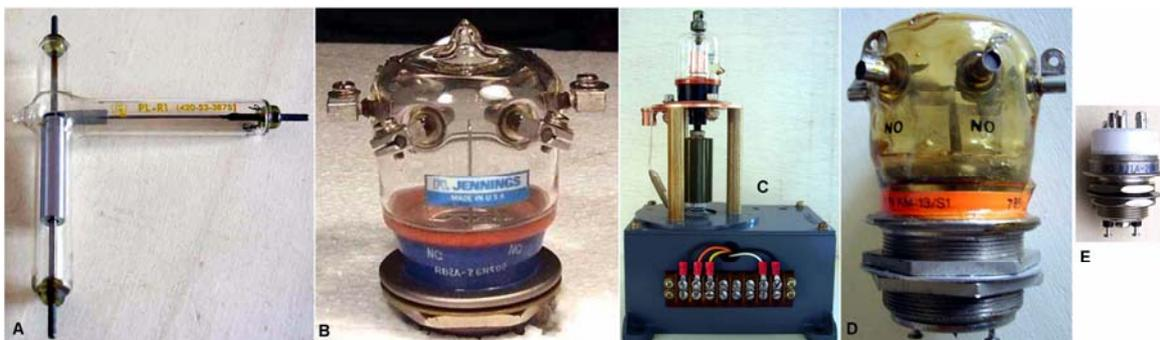
Fig. 12.2 - Vacuum relays. A) [PL-R1](#) and the many equivalents, as [5TA-75](#) and Eimac [VS-2](#) were rated for 20 kV at 7.5 A up to 15 MHz and 5 A up to 30 MHz. B) [RB2A](#) DPDT relay is rated for 20 A at 20 kV. The coil is in the screw mount base. C) [R5C4304](#) is a high-power contactor capable of switching up to 50 A at 40 kV. D) [KM13-S1](#) is a gas filled DPDT relay, used for handling the discharge of capacitors, E) [RJ1A](#) is a modern ceramic relay rated for 3.5 kV at 18 A.
