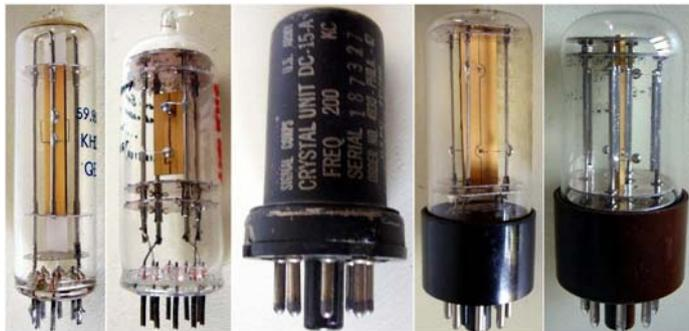
**Fig. 12.5 – Samples of precision quartz crystals, all vacuum sealed to prevent the oscillation damping due to the atmosphere.**
