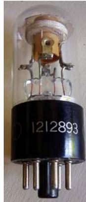
Fig. 12.1 - A sealed coil, the 1212893 made by General Electric, was used in the local oscillator of some Crosley car radios. Vacuum sealed tuning components, inductors and capacitors, were commonly used in aircraft and in military equipment to protect them from dust, moisture and condensation.
