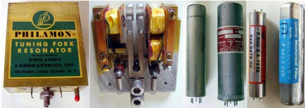
Fig. 12.6 – Samples of tuning forks, used to precisely control oscillations at very low frequency, typically up to about 1 KHz. The latest photo shows a couple of Collins mechanical filters, used as very high Q filters in the IF sections of AM receivers.
