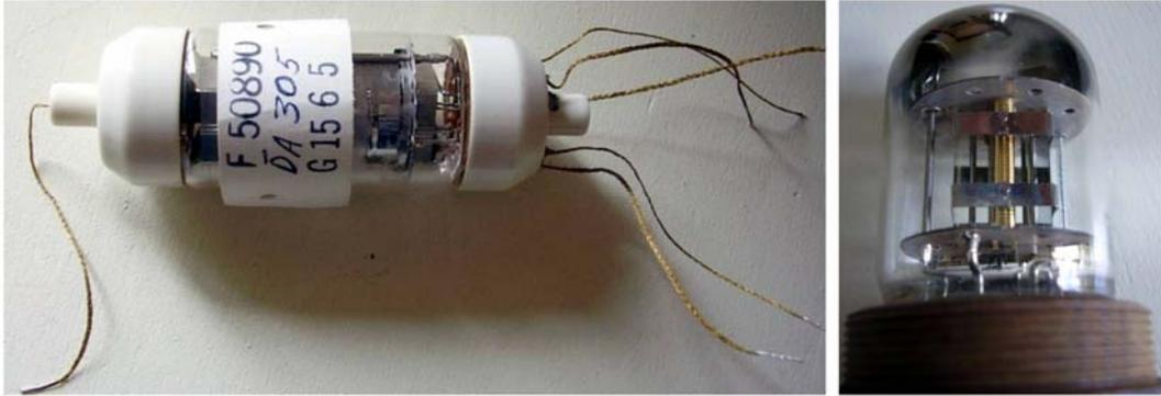
Fig. 11.3 - The Bell 175HQ, used in the transatlantic telephonic system TAT and its successor, the 455A.
