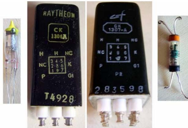
Fig. 11.8 - Samples of vacuum tubes specifically designed for weapons. From left, a [2D29](#) subminiature thyratron used in the T-172 proximity fuze, Raytheon [CK1306A](#) and [CK1307A](#), believed to come from the active sonar search head of early Mark 44 torpedoes, and the NEC [M-999](#) thermal cutoff, used as SAD in a torpedo guidance board.
