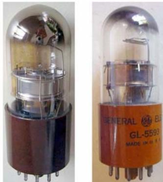
Fig. 11.1 - The collection includes both the types made by General Electric, [2H21](#) and [5593](#).
