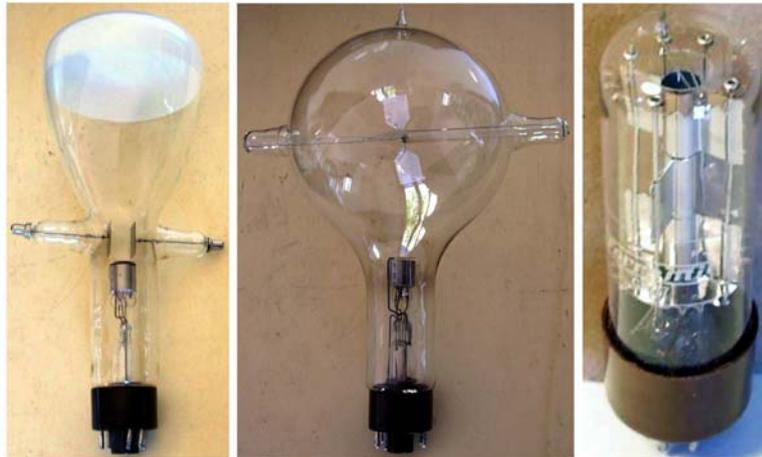
Fig. 11.4 - These tubes were quite common in the physics laboratories of technical schools in the twentieth century. From left, a [BR-2](#) Braun cathode ray tube, an [SKR-2](#) electron-flow windmill and a [GRD7](#) symmetrical temperature-limited diode.
