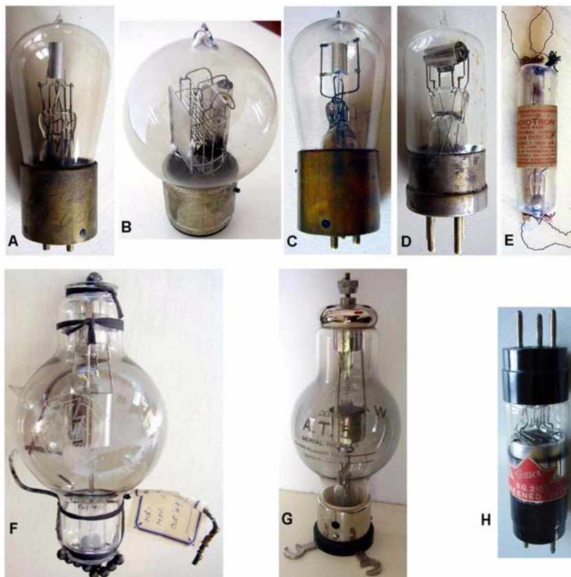
Fig. 2 - Early tubes from the Great War to the twenties. A - General Electric VT-14 general purpose amplifier, about 1917-1918. B - Western Electric VT-2 triode delivered to Signal Corps from 1917. C - General Electric TB1 kenotron or diode, about 1918. D - Philips D-II detector or amplifier, around 1921, still retaining the horizontal electrode arrangement of the French TM. E - The Audiotron from Cunningham was sold from the mid 1915 in the single filament version. The double filament version, as the one in the collection, was advertised in August 1916. F - MRI , a British power rectifier in use from early 1919. G - The A.T.50 was a very fine power transmitting triode made around 1920. H - This Cossor S.G.210 is one of the double-ended screen grid tubes appeared around 1927. (Click the image to enlarge)
