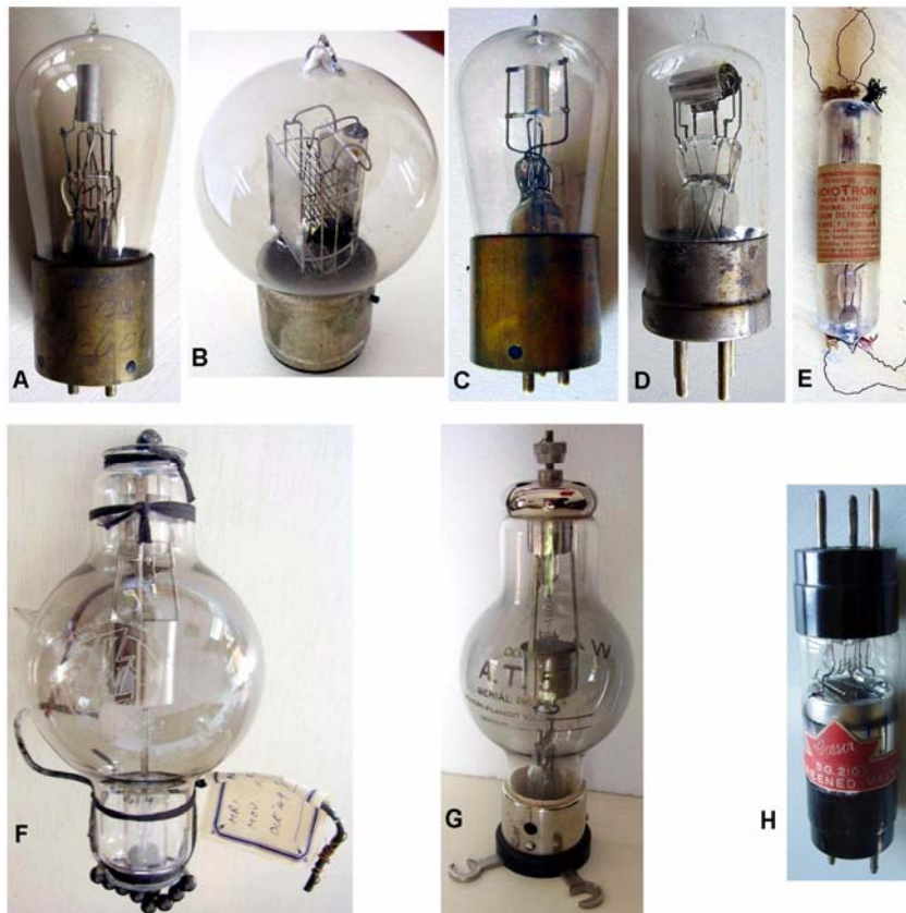
Fig. 2 - Early tubes from the Great War to the twenties. A - General Electric VT-14 general purpose amplifier, about 1917-1918. B - Western Electric VT-2 triode delivered to Signal Corps from 1917. C - General Electric TB1 kenotron or diode, about 1918. D - Philips D-II detector or amplifier, around 1921, still retaining the horizontal electrode arrangement of the French TM. E - The Audiotron from Cunningham was sold from the mid 1915 in the single filament version. The double filament version, as the one in the collection, was advertised in August 1916. F - MR1 , a British power rectifier in use from early 1919. G - The A.T.50 was a very fine power transmitting triode made around 1920. H - This Cossor S.G.210 is one of the double-ended screen grid tubes appeared around 1927. (Click the image to enlarge)
