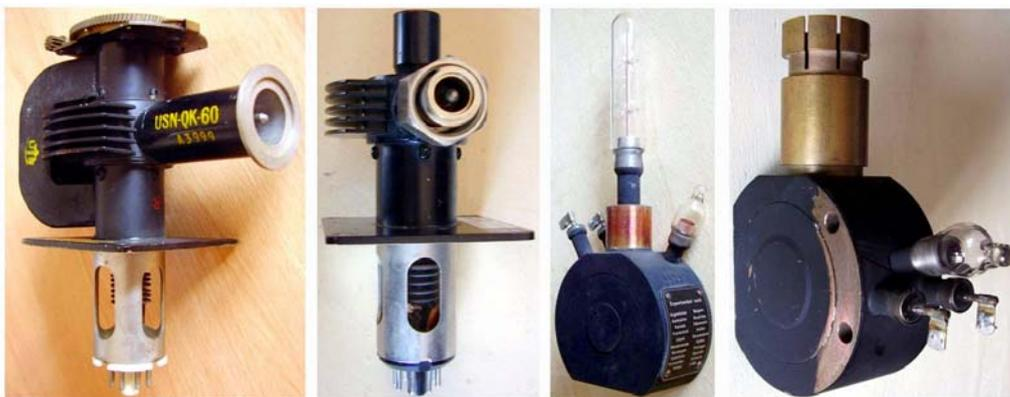
Fig. 6.6 – Some CW magnetrons. Even if the tunable [OK-60](#) (a) is given for pulsed operation, it can be operated at any pulse length and repetition rate. It is similar to the fixed frequency [5609](#) (b), 70W output at 2450 MHz, intended for RF heating. Both probably derived from the experimental CW type CM16B described by Collins. The German [MG8/200](#) (c) is capable of delivering 250W at 2.42 GHz, while [MG20](#) delivers 50 W at 5.8 GHz.
