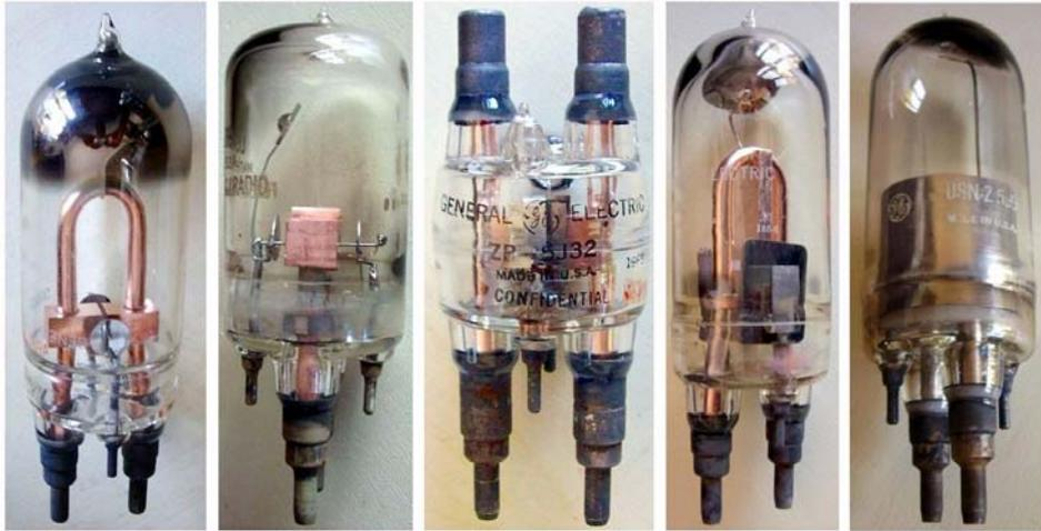
Fig. 6.7 – Split-anode CW magnetrons were designed during WWII to operate as RF sources for jammers in the VHF-UHF bands of German radar sets. The collection includes the four types gone in production, plus an experimental type, all described in Very High Frequency Techniques, volume II, by Radio Research Laboratory of Harvard University.
