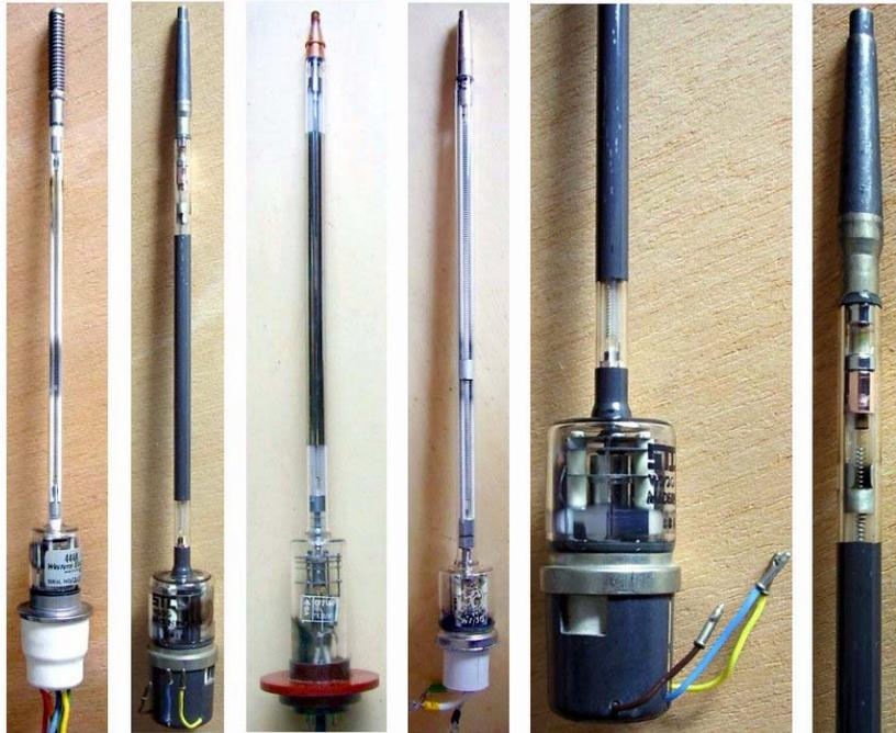
**Fig. 6.9** – Pictures of some TWT tubes made by Western Electric and by British Standard Telephone (STC), with details of electron gun, of helix and top termination. The electron beam travels inside the helix and must be kept focused by a magnetic field generated either by a permanent magnet or by a focusing coil, depending upon the actual type.
