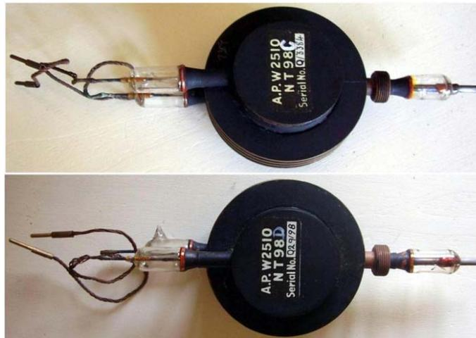
Fig 6.8c - Early British magnetrons directly derived from E1189 prototypes, [NT98C](#) and [NT98D](#), later approved as CV1494. These types too are still unstrapped, with output power lower than 10 kw peak at 3 GHz.
