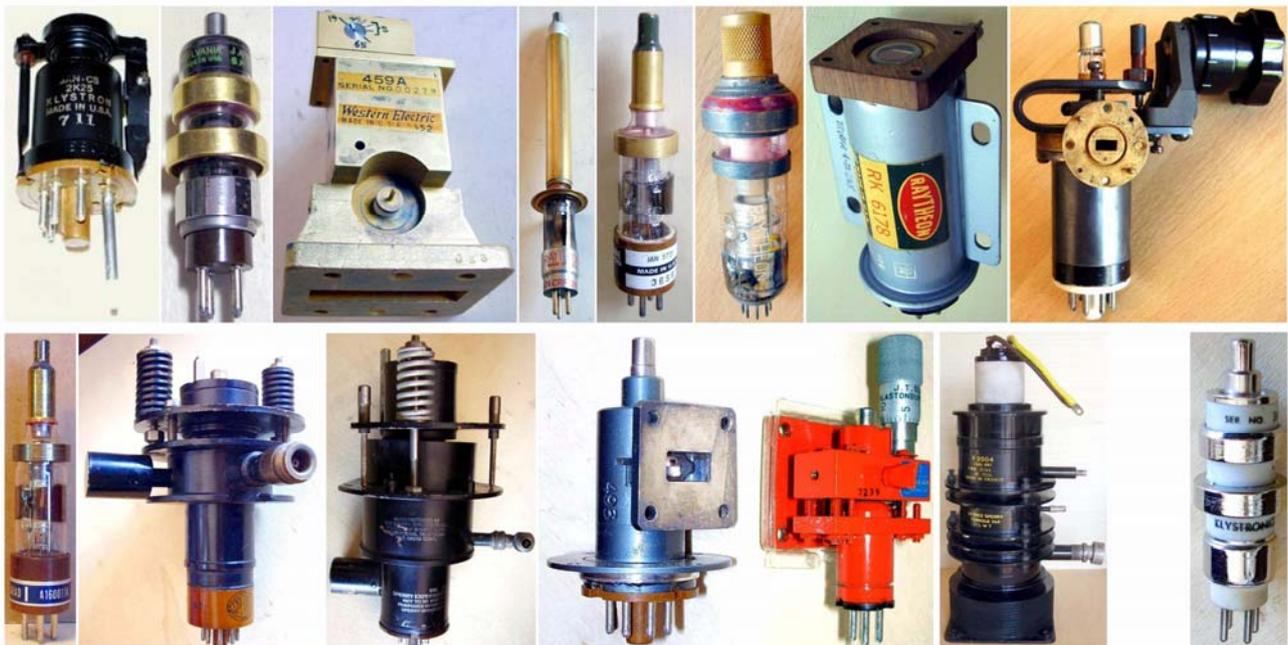
Fig. 6.3 – Shapes of some U.S. klystron tubes
