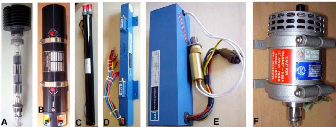
**Fig. 6.10** – Some more TWTs: (A) and (C) require external focus coils. (E) and (F) are BWOs.
