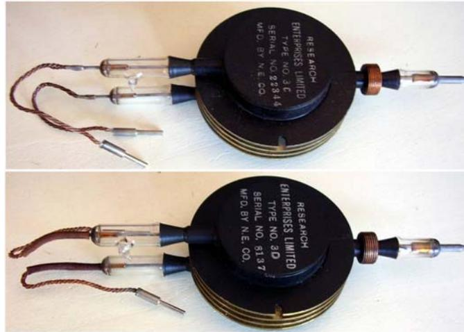
Fig. 6.8b - Canadian [REL3C](#) and [REL3D](#) are copies of the very early E1189 serial no. 12, brought in America by the Tizard mission in 1940. Still unstrapped, they operated around 3 GHz, with a peak output power in the order of 10 kW.
