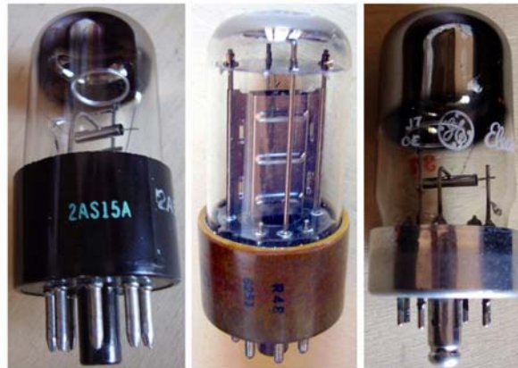
Fig. 8.1.1 – Current limited diodes used in power supply current stabilization circuits.
