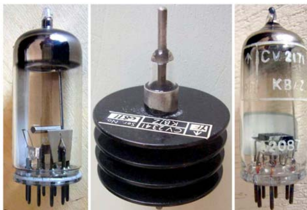
Fig. 8.1.2 – Some current limited diodes designed for use as noise generators. The CV2341, in the middle, was designed to be directly interfaced to a 75 ohm coaxial line.
