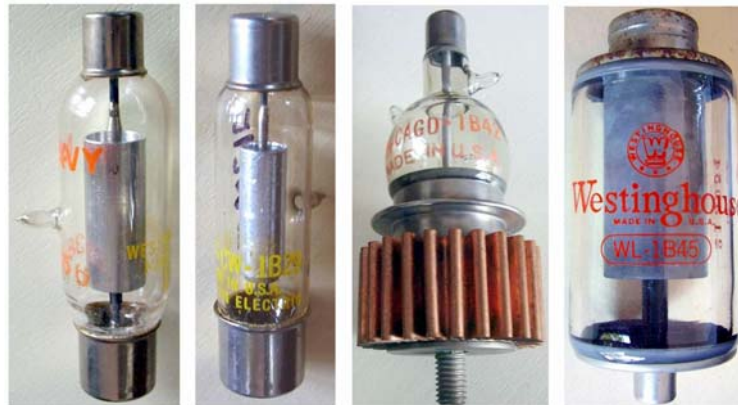
Fig. 7.2 – Some two-electrode spark gaps. From left, the popular 1B22 and its smaller variant 1B29 , 30 A peak current, the iron-sponge mercury cathode 1B42 and the 1B45 , 450 A peak.
