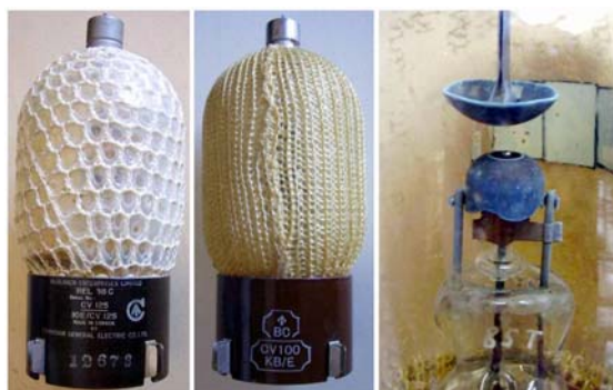
Fig. 7.3 – Two trigatron tubes, the second one from Canadian REL, and detailed view of the internal spark gap, with the trigger electrode tip just visible in the middle of the cathode dome, its stem being covered by a glass tubing, protruding from the bottom press.
