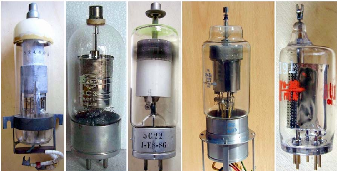
Fig. 7.8 – Thyratrons for radar pulsers. The first one is a British mercury type CV22 . Other are hydrogen thyratrons, the third and the fourth with titanium-hydride reservoirs. The latest one is a small thyratron in a miniature glass envelope, yet capable of switching 20 amps at 1.2 kvolts.
