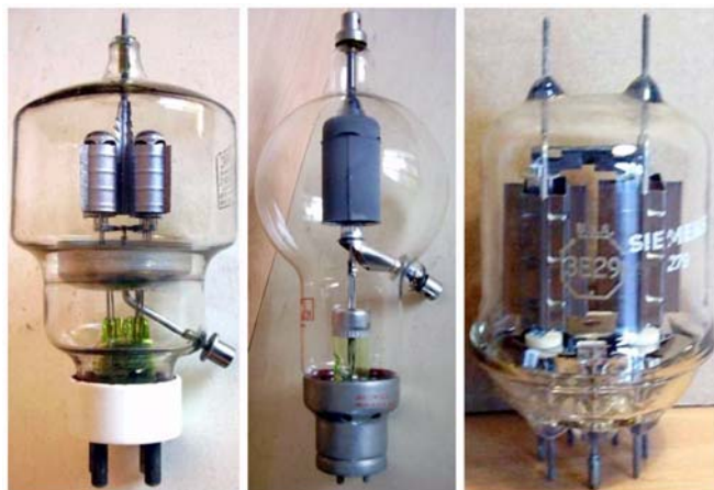
Fig. 7.5 – Some tubes used as switches in radar pulsers and derived from transmitting types. From left, the VT-129 (304TL) was designed, assembling four electrode packs of the 75TL transmitting triode. The 6C21 in the middle actually is a 1000T, specified for higher filament voltage, in order to grant the required emission. The 3E29 dual tetrode was derived from the transmitting 829 , replacing ceramic spacers for the previous mica ones, to prevent arcing at high voltages.
