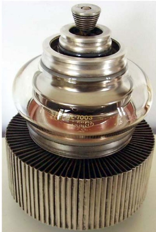
Fig. 7.7 - Two high-power tubes designed for pulse switching applications. The ML-7003 is a shielded grid triode capable of operating at 40 kV, 80 A peak. The AX-10318 is a tetrode capable of operating at 100 kV.
