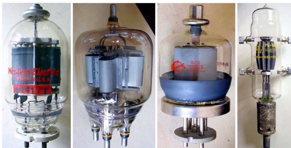
Fig. 7.6 – Tubes specifically designed for pulse modulators are characterized for their high cathode surface, their excellent insulation and often guard rings to prevent corona discharge. Here from left a 5D21 , with four in-line cathodes, a 701A , with four electrode sets of 350A, and a 4PR60B . Probably the PL-185/527A , even if used in the VHF ring oscillator of the radar AN-TPS-18, was also one of the largest tube used as hard pulser, being capable of handling pulses of 60 amps at 30 kvolts.
