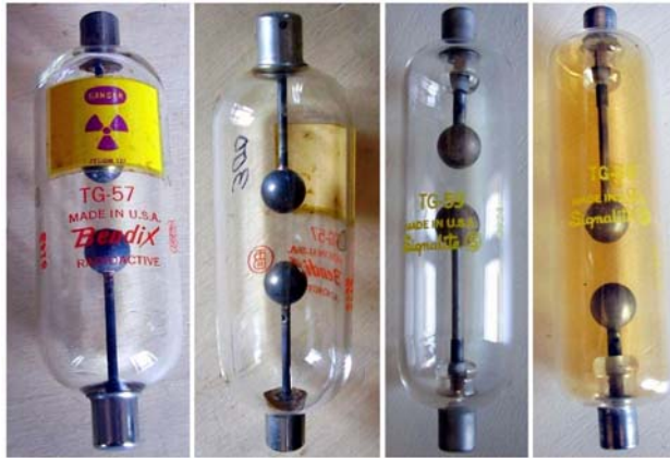
Fig. 7.4 – Protective spark gaps, used to prevent excessive high-voltage build-up in radar modulators. Sealed construction and some radioactive activators are used to grant predictable trigger voltage, regardless of the environmental conditions, temperature, pressure or moisture.
