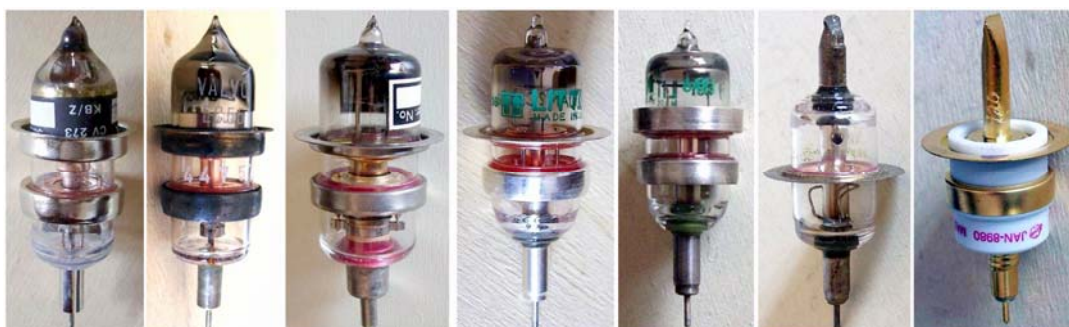
Fig. 5.8 – An overview of European and American rocket tubes. Starting from left, the early type, the CV273 from GEC, the EC55 from Philips, a later GEC larger power variant, the CV397 . The next four tubes are American designs, including the basic 2C36 , the folded grid, folded anode rings 6481 , the discoidal grid 5768 , also proposed as UHF television preamplifier, and the latest cermet variant, the Eimac 8980 , built in the eighties as replacement for the discontinued glass-bulb 2C37 .
