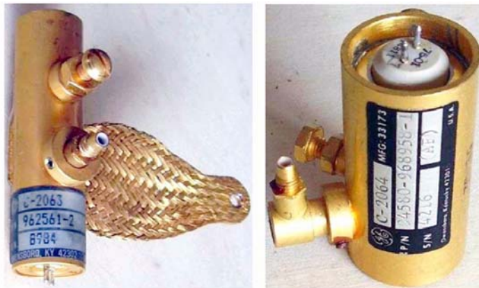
Fig. 5.15 - For specific microwave applications, due to the difficulties for average customers in manufacturing, assembling and tuning their own cavities, some tube manufacturers offered standard modules, built around pencil or cermet tubes. Typical applications included radiosonde transmitters, radio altimeters and other avionic equipment. The huge quantity of gold all over the surfaces of these two GE modules used in the radioaltimeter of licence built F-104G interceptor well gives an idea of their cost.
