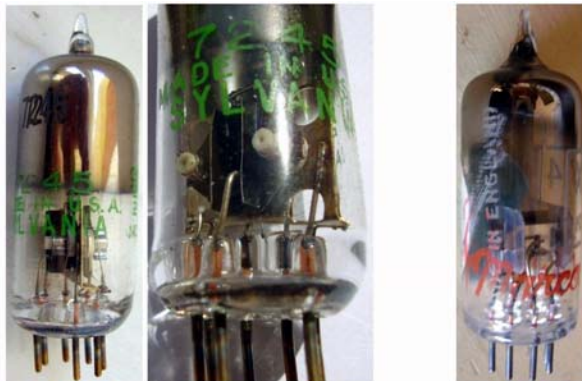
Fig. 5.16 - Even miniature glass envelopes were used for planar triodes intended to operate at frequencies under 1000 MHz. The first two images refer to the Sylvania 7245 , equivalent to 6J4, while the last image refers to the British Marconi A1714 , approved as CV408, capable of operating as low-noise amplifier or oscillator up to 1000 MHz. 7245 planar structure was also proposed in a ruggedized ceramic enclosure, engineered for fully automatic production.
