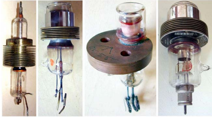
Fig. 5.6 – Some micropup tubes. From left, the Amperex 8011 , one of the many American replacements for the British V.T.90 , used in pulsed operation up to 300 MHz. The British CV92 , also made in United States and in Canada with different codes. The CV55 , capable of operation at 600 MHz. The Canadian REL 4C29 , an improved variant of the CV92.
