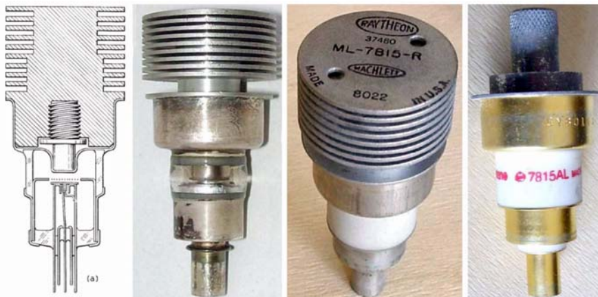
Fig. 5.10 – Left to right, section of the GE experimental L-14, a 2C39 , a ceramic variant, the 7815R , and a gold-plated conduction cooled 7815, selected for airline use.
