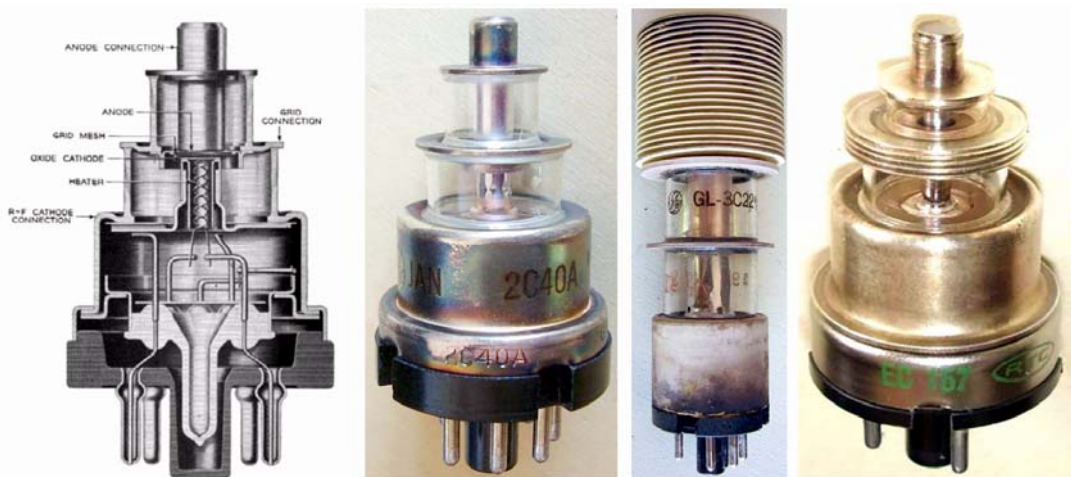
Fig. 5.9 – From left: the section of a 2C40 and the tube itself, a 3C22 capable of 125W plate dissipation and the EC157 , one of the few European lighthouses, used in UHF radio-relays.
