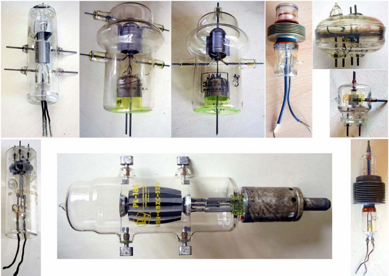
Fig. 4.6 - Shapes of some transmitting power tubes introduced during WWII or few years before and designed to operate from VHF to UHF bands. The tube in the middle of the bottom row was used as VHF oscillator but also as high-power pulse modulator in radar applications.
