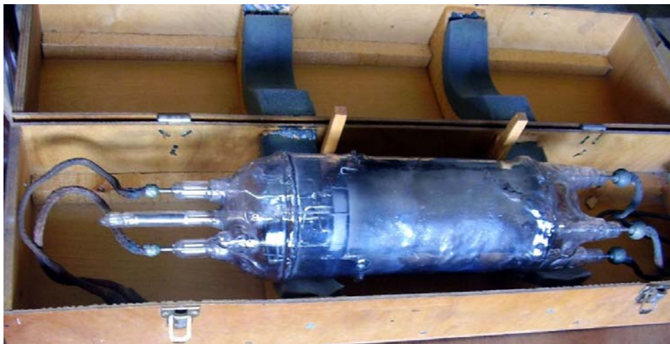
Fig. 4.5 - One solution to reduce envelope size in high-power tubes was the use of silica, capable of withstanding temperatures in excess of 1000 degrees, introduced by Mullard since 1918. Here a TYSS5-2000 .
