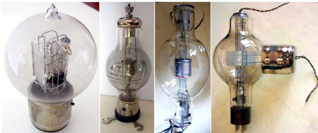
Fig. 4.1 – Some of the very old transmitting tubes, from the Great War to the early '30s.
