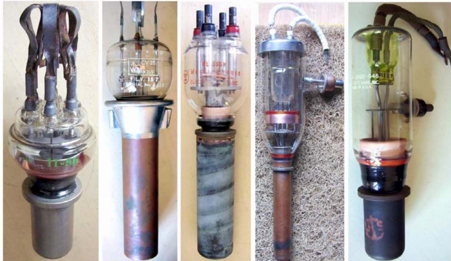
Fig. 4.4 – Higher power could be handled by water cooling. A water-jacket heat exchanger hosts the tube, usually the copper anode being mounted upside down.
