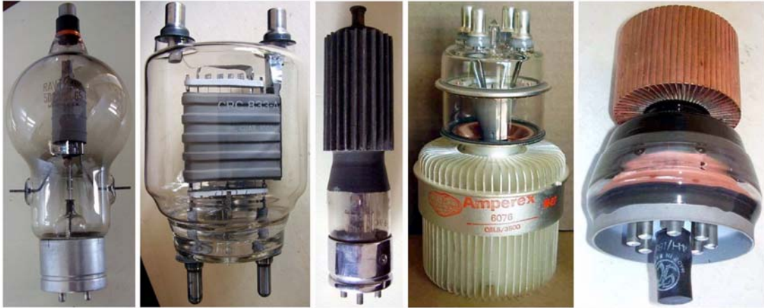
Fig. 4.3 – Increasing power, more efficient heat radiators were required. Carbonized or tantalum anodes help to operate at higher temperature, also improving radiation cooling. External anodes, made of copper sealed to glass spacers even with finned surfaces cooled by forced-air flow, were introduced to increase cooling.
