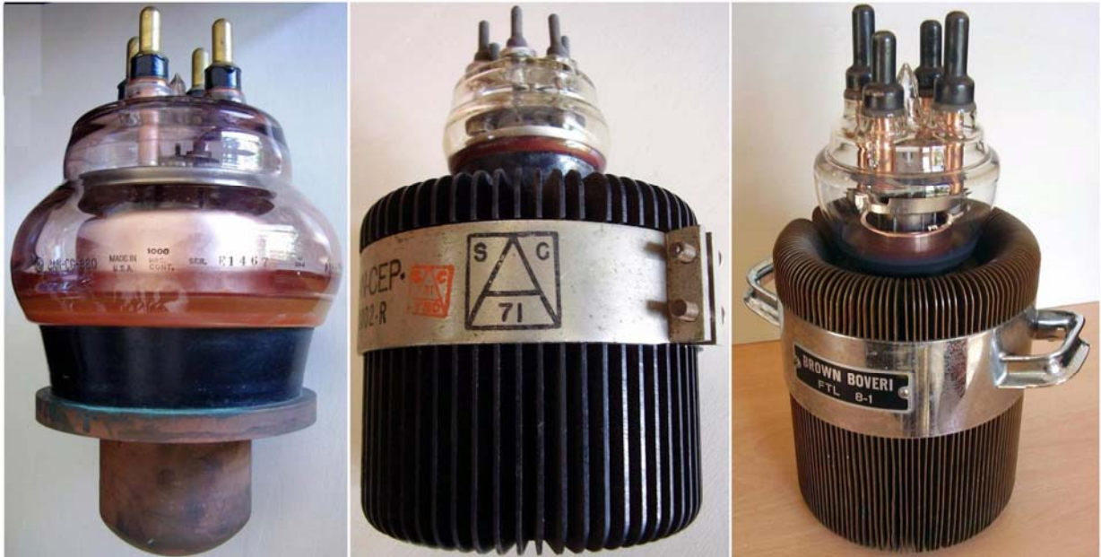
Fig. 4.8 - Other examples of power transmitting tubes. The first one, a GL-880 is a water-cooled type with folded anode. The one in the middle is a compact 8002-R , while the third sample is a quite heavy FTL 8-1 , 8 kW forced-air-cooled triode.
