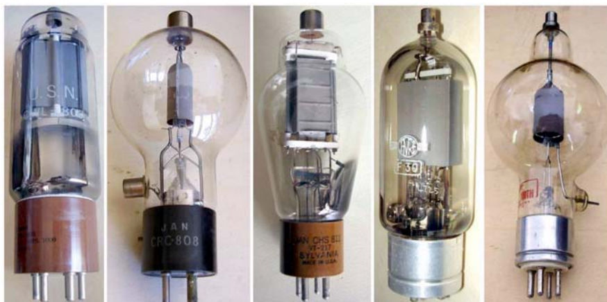
Fig. 4.2 – Some of the low to medium power, convection-cooled transmitting tubes.
