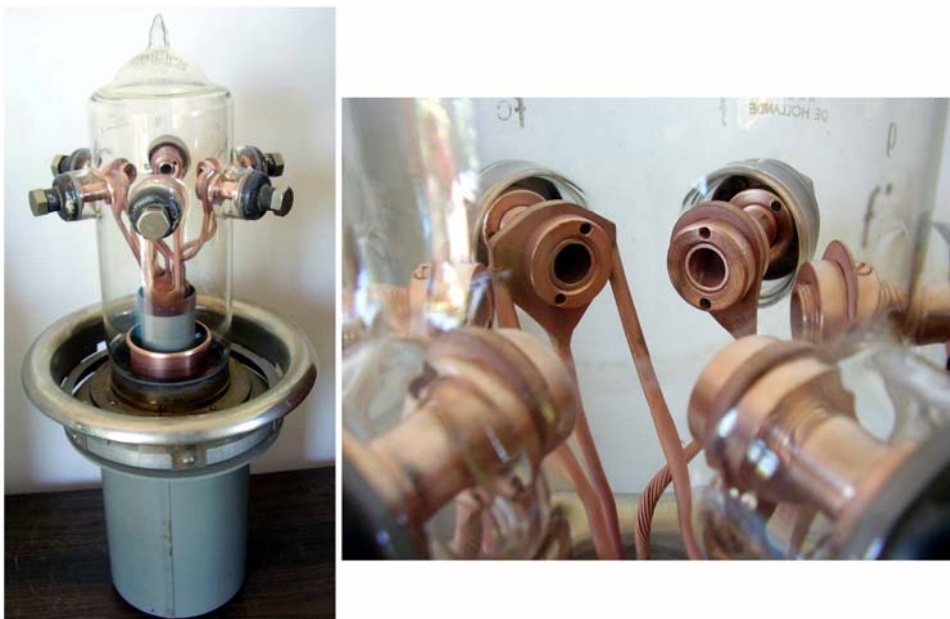
Fig. 4.7 - This TAL 12-35 is a true masterpiece, where most advanced solutions of glass-to-metal sealing were used to carry high operating currents, also granting the proper insulation.
