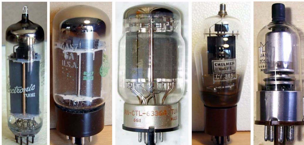
Fig. 3.2.3 – Several power tubes were intended to operate as series or parallel active control devices in DC voltage regulating circuits.
