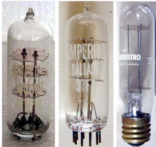
Fig. 3.2.2 – A tiny iron wire in hydrogen atmosphere was used to stabilize the current into an external load, even under wide supply voltage variation.
