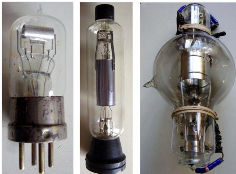
Fig. 1.4 - Other interesting vacuum tubes which can be dated around 1920, the Philips D-II triode (1921-1922), the Telefunken RS19 transmitting triode (about 1919) and the British MOV VT30 power triode (1922).
