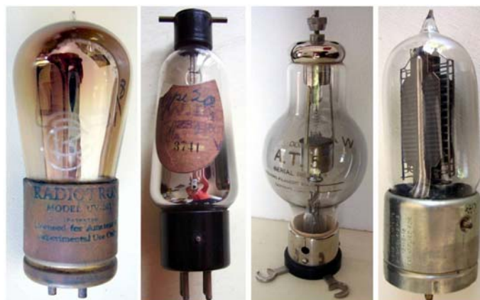
Fig. 1.2 – Tipped bulbs were in use in the first half of the 1920s. Early types for AC operation were sometimes characterized by heater connection from the top, to facilitate the cabling in the upgrade of old battery sets. The third tube from left is one beautiful WWI British transmitting type, shown close to a WE VT-1 of the same years.
