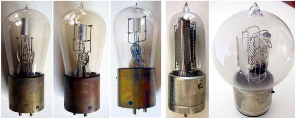
Fig. 1.3 - American military tubes used during WWI. One of the early triode made by General Electric for Navy and Signal Corps, the CG-1162 / VT-14, was modified with four plate supporting tabs to better withstand shocks and vibrations. The same structure was used in the TB1 diode. Western Electric used frame grids, ribbed plates and a glass arbor to stiffen its military tubes.
