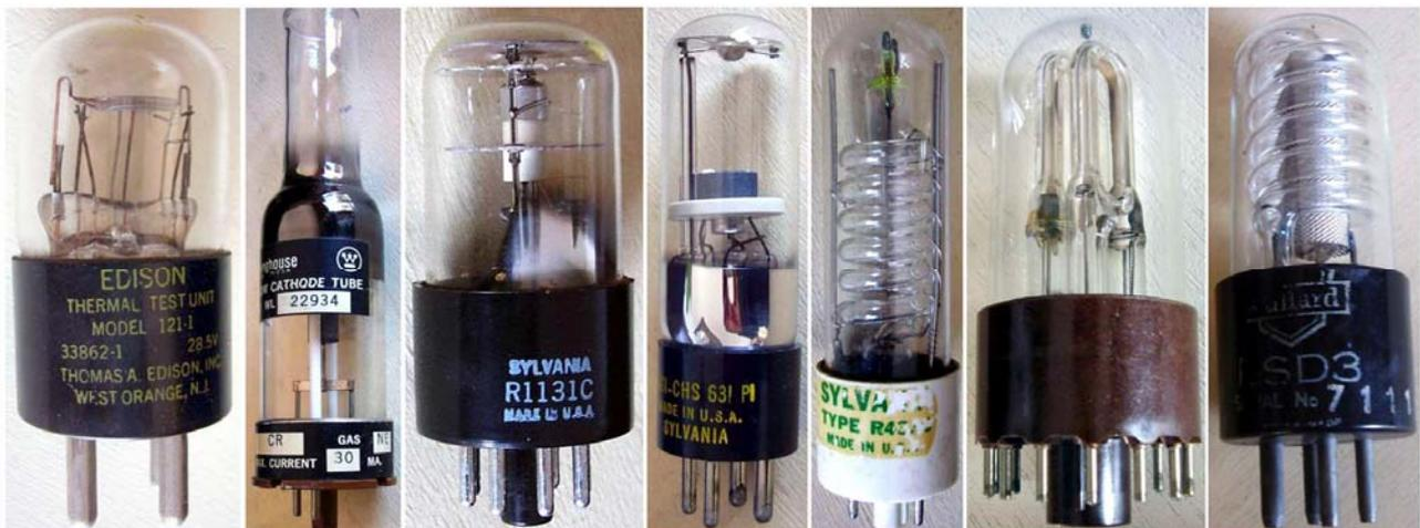
Fig. 8.9 – Samples of different radiation sources. From left we see a thermal test bulb, a hollow cathode monochromatic light source, a crater lamp, used to generate the tiny scanning beam in the early facsimile sets, and four stroboscopic light sources.
