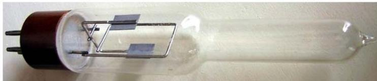
**Fig. 8.10.4 - The Philips CIG22 is a cold cathode Penning sensor.**
