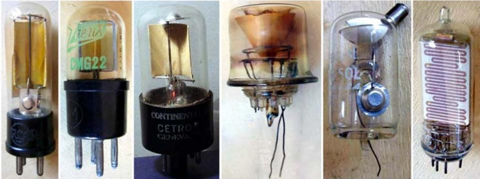
Fig. 8.8.1 – Standard and custom photocells. The last device is a cadmium-sulphide photoresistor.
