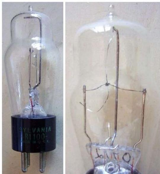
Fig. 8.10.2 - The Sylvania R1100 is a thermocouple type vacuum sensor.
