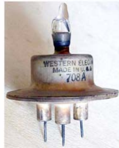
Fig. 5.12 - This very unique design appeared around 1940 to operate as grounded-grid amplifier/mixer in L and even in S-Band radars.
