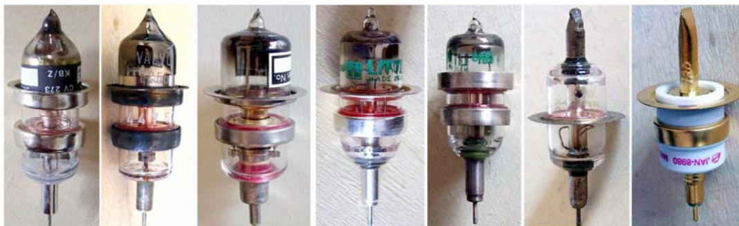
Fig. 5.8 – An overview of European and American rocket tubes. Starting from left, the early type, the CV273 from GEC, the EC55 from Philips (Valvo), a later GEC enlarged power variant, the CV397. The next four tubes are American designs, including the basic 2C36, the folded grid, folded anode 6481, the discoidal grid 5768, also proposed as UHF television preamplifier, and the latest cermet variant, the Eimac 8980, built in the eighties as replacement for the discontinued glass-bulb 2C37.
