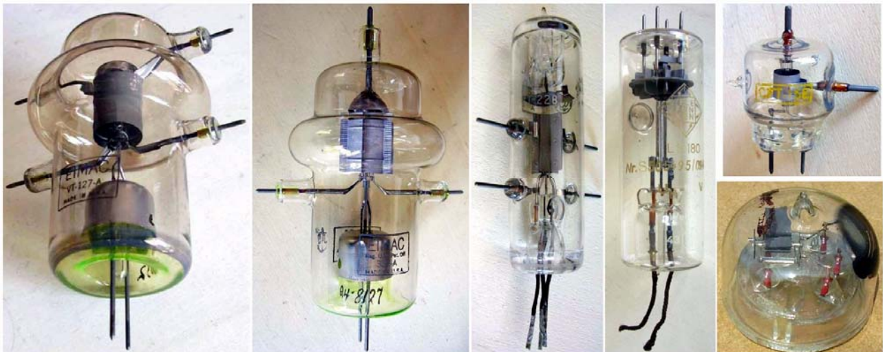
Fig. 5.4 – Some VHF/UHF transmitting tubes were designed to be mounted as direct extension of the associated resonating line.
