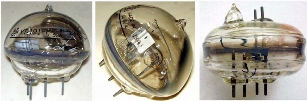
Fig. 5.3 – Left, two views of a VT-191 ‘door-knob’ single-ended UHF transmitting triode. Right, a WE 368A, with anode and grid connections both from base and from top.
