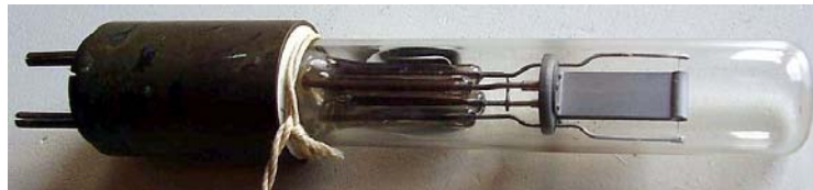
Fig. 5 - Siemens RM4025 looks to be a split-anode magnetron with self-contained resonating system. It was designed for operation at 3 cm. Still in evaluation phase at the end of the war. Click on image to enlarge.
