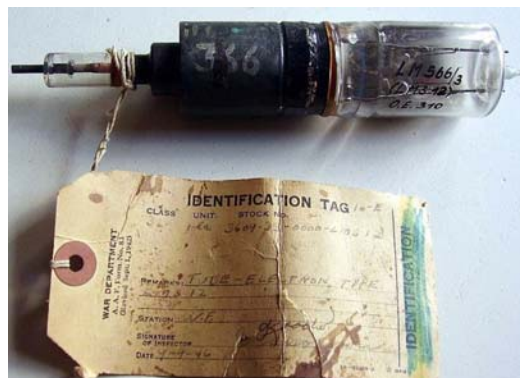
Fig. 3 - This is the only known sample of LMS 12 . On the glass bulb also its experimental code, LM 566/3, is well visible. It still retains the US War Department classification tag, dated 1946. The rod on the left looks to be the center conductor of the coaxial output. The two heater/cathode pins are on the right of the large glass bulb. Click on the image to enlarge.
