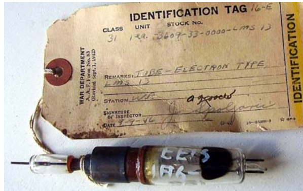
Fig. 4 - LMS 13 sample still retaining its US War Department classification tag, dated 1946. 5 kW at 1.625 cm wavelength. 18-resonator anode system. Click on image to enlarge.
