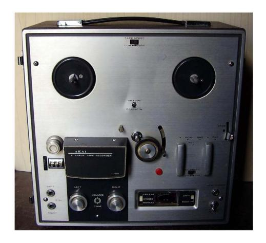
4-track, three-speed tape deck. Pole switching of the capstan motor windings, to operate at either 50 or 60 Hz frequency. 40 to 18,000 Hz at 19 cm/s.
