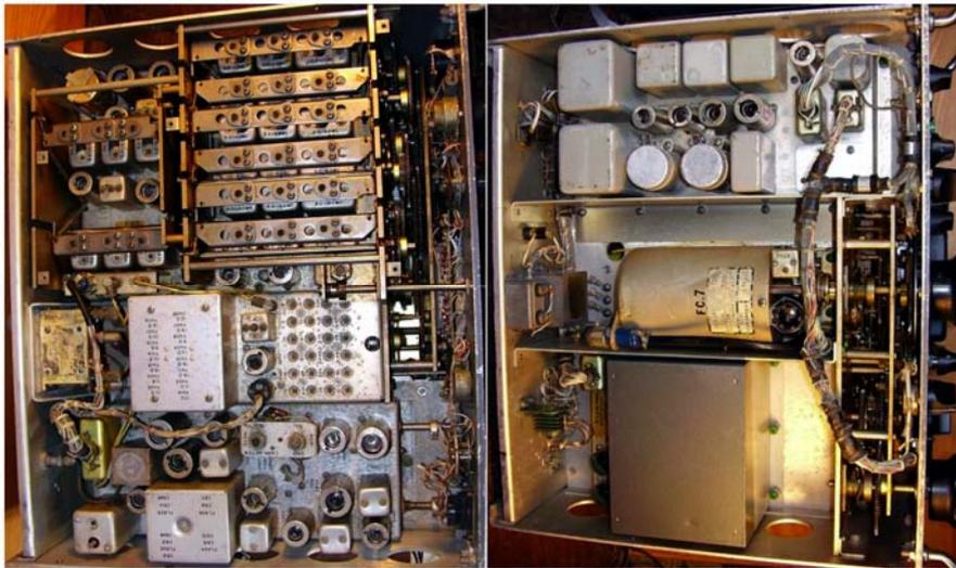
**Fig. 2 – Two views of the inside arrangement. Left, on the upper side of the frame we see the RF and variable IF, the crystal oscillator and the fixed IF modules. Right, the AF, the PTO and the power supply modules are visible under the frame.**
