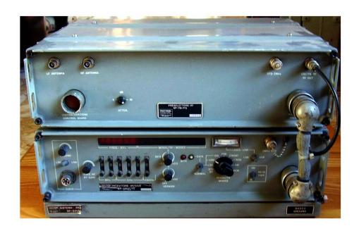
The Elmer SP-841/D is a high-performance communication receiver system. It features voice/data operation and interoperability in Link-11 ntds data system. It can be remotely controlled by use of a remote control set.
