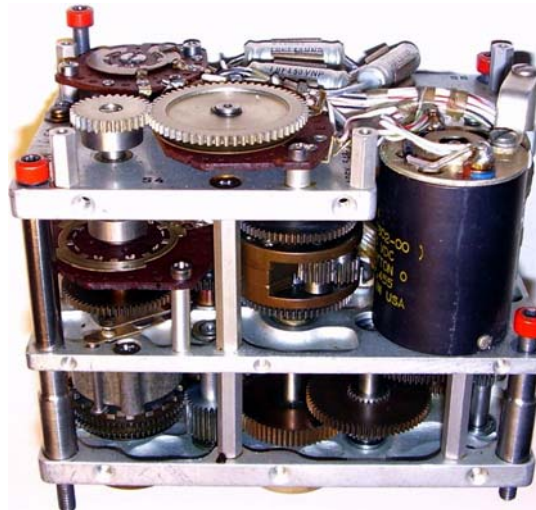
Fig. 11 - The tuning power drive module of the ARC-51 with the DC motor on the right. Movements are propagated to other subassemblies by a gear train in the supporting base.
