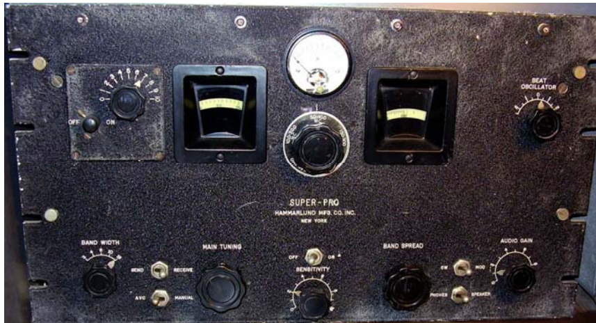
Fig. 5 - Hammarlund SP110 'Super Pro' was one of the best pre-war receivers. It could operate up to 20 MHz in five bands to custom specifications. Tuning was made easier by the band-spread dial and by the S-meter placed just over the band switch. In this sample we see the crystal filter installed, the small panel on the left of the main tuning dial. This receiver is completed by an introductory article from Jan. 1938 Electronics and its manual.
