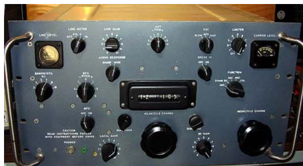
Fig. 8 - Front view of the R-390A, showing the two large tuning knobs, for fine tuning and for megacycle band switching and the mechanical digital readout in the middle.
