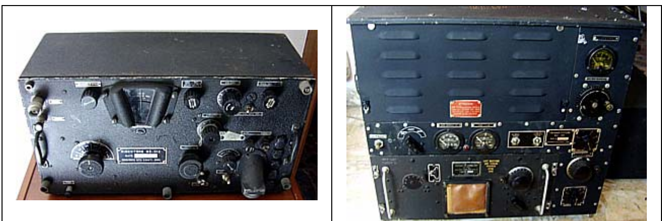
Fig. 6 - Left, BC-312 and the AC operated version BC342 were among the most advanced receivers designed before the war and built in hundreds of thousand units during WWII. It was a 9-tube superheterodyne operating from 1.5 to 18 MHz over six bands. 470 kHz IF frequency with additional crystal filter. Right, BC-191 was the most common liaison transmitter during WWII. With the proper tuning plug-in, lower-left in the above image, it could operate from 200 kHz to 12.5 MHz both in CW and in AM.
