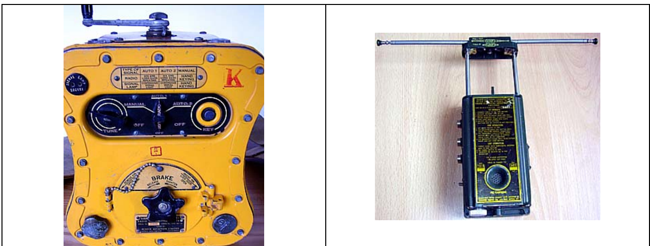
Fig. 10 - Left the BC-778 'Gibson Girl' for its shape was the first survival transmitter given to US aircraft pilots during WWII. Right, the RT-159/URC-4 with antenna in operating position was in use in the Vietnam War.
