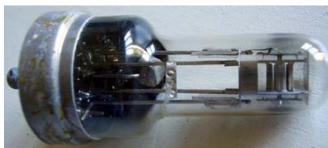
Fig. 7 - The GEC magnetron CV79 used as microwave source in the British Wireless Set No. 10.
