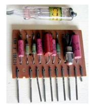
I also found some additional examples of computers, or computer related peripherals, in which subminiature tubes were used. Anyway they refer to analog interfaces, building blocks and to airborne computers, rather than to digital mainframes. Also dedicated equipment took advantage of the reduction of power and space offered by subminiature tubes in their logic circuits, as in the case of this <u>KWR-37</u> ciphering equipment
