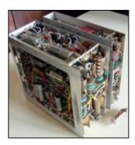
Another application using 5703 subminiature triodes in the A to D peripheral interface built by Boeing was described in this article from Electronics, August 1954.
