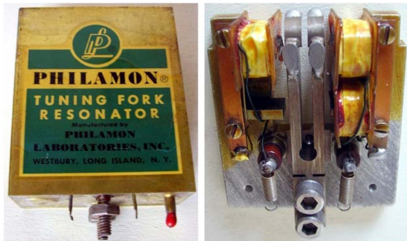
Fig 2 - A 1350 Hz sealed tuning fork resonator used as frequency reference in the timing generator of a TACAN ground beacon transponder. On the bottom right of the unit well visible is the exhaust hose with sealed red tip. Right the same unit open, to show the fork, the single pick-up coil and the two drive coils close to the right tine. On the top of both tines there are the tuning and balancing masses, part of them supported by the two right angle reeds. To reduce acoustical coupling, the coils are connected to the pins of the case by the two spring wires visible aside the fork, near to the bottom. The unit was originally mounted on rubber spacers. Dimensions are 55 x 68 x 25 mm; weight is 240 grams.
