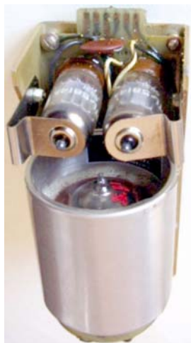
Fig. 11 – Photo of a 100Kc decade counting module with a BD301/6703 trochotron.
