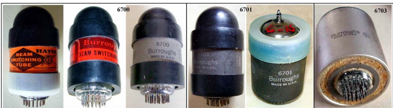
Fig. 4 - From left: three samples of 6700, the first one badged Haydu, two samples of 6701 and a 6703.
