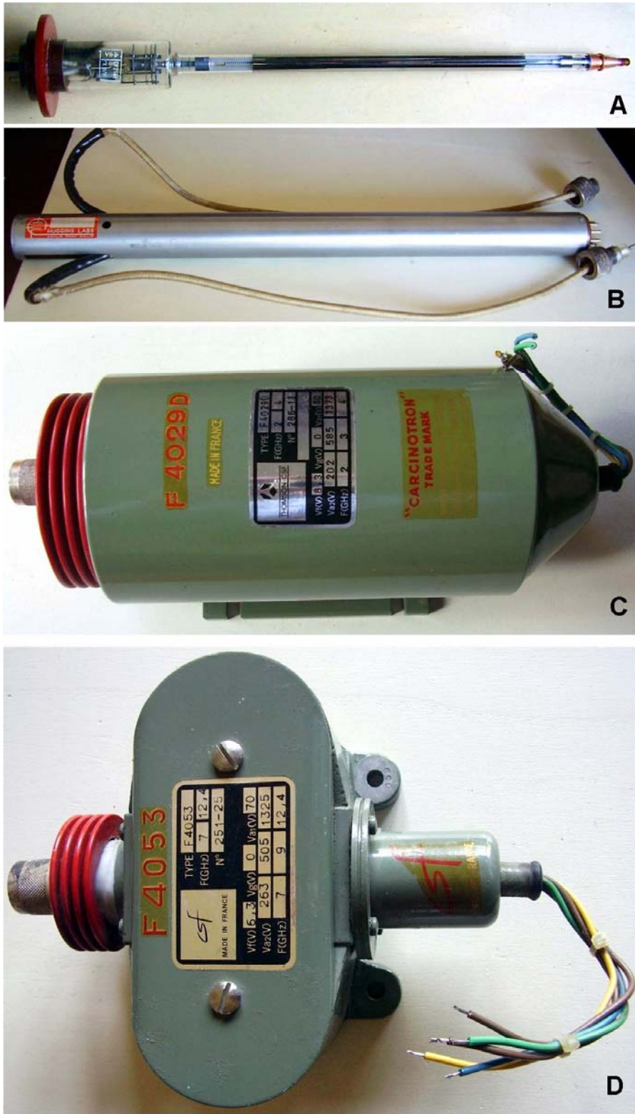
Some TWT and BWO tubes: A) The bare STC W72D TWT amplifier. B) The Huggins HA2-HP helix coupled amplifier. C) The CSF F4029D BWO, also referred to as Carcinotron 'O'. D) Another CSF carcinotron was this F4053 .
