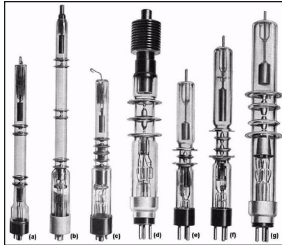
Fig. 1.4 – Linear beam klystron tubes developed by Bell Laboratories. 4(a), 4(b) and 4(c) are very early prototypes developed prior to WWII. 4(b), 4(f) and 4(g) are cascade types.
