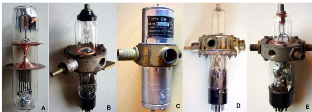
Fig. 1.7 - The story of early British reflex klystron from summer 1940 to the end of 1941. A) An unbased early sample of ' Sutton tube ' likely built at the Bristol Signal School. B) A sample of NR89 , with the Air Ministry code 10E/501. C) In 1941 Rogers was asked by Canadian REL to design ruggedized copies of NR89 for its microwave radar sets. The Type 8 is similar to the 'Sutton tube' with an aluminum shell and an improved tuner. D) At the end of 1941 EMI introduced an improved and more stable design which originated some frequency variants, as this CV35 . E) Knowing that Western Electric had introduced the 707A low-voltage reflex klystron, in late 1941 TRE asked EMI for developing a similar device. This 10AL1 is an experimental prototype, built to evaluate a better coupling of the resonator to the electron beam and the generated noise. The design will lead in 1942 to the introduction of a new family, including among the others the CV238 , with meshes of corrugated tape brazed to the internal rim of the resonator discs.
