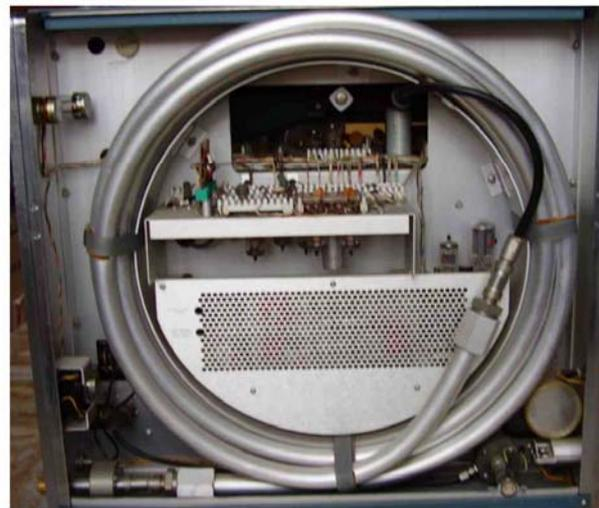
This huge oscilloscope was introduced in the early sixties, with very unique features. Vertical bandwidth from DC to 1000 MHz minimum at 3 dB and risetime less than 0.35 ns were claimed, thanks to its distributed deflection type CRT.
