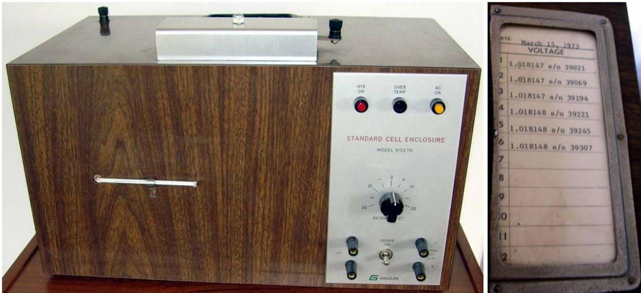
The Weston cell was first devised in 1893 and accepted as primary voltage standard since 1911. Still today it is in semi-clandestine use to check solid state voltage references. Due to environmental restrictions for its major components, mercury and cadmium, its use is very limited and secret today. Unfortunately, even the documentation and the same datasheets have been removed from the Web, probably fearing mercury contamination of the keyboards!
