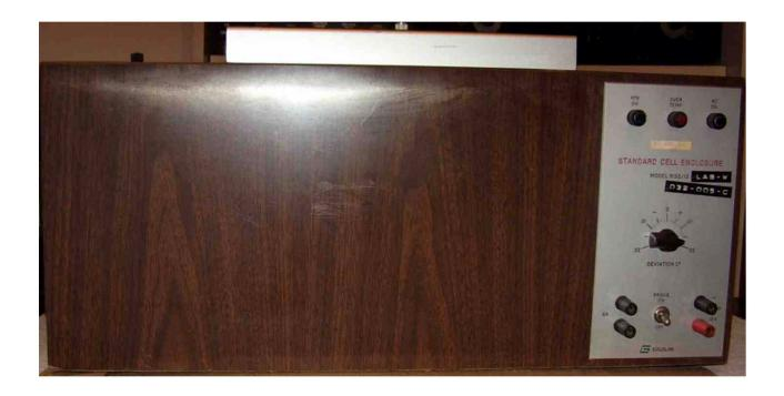
The Weston cell was first devised in 1893 and accepted as primary voltage standard since 1911. Still today it is in semi-clandestine use to check **erratic solid state voltage references**. Due to environmental restrictions for its major components, mercury and cadmium, its use is very limited and secret today. Unfortunately, even the documentation and the same datasheets have been removed from the Web, probably fearing mercury contamination of screens and keyboards!
