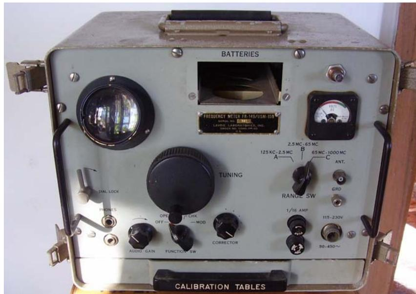
The heterodyne frequency meter FR-149/USM-159 can be considered the solid-state version of the well known SCR-211/BC-221. The sample in the collection was made by Lavoie Laboratories to a 1963 order. Looking at the components used inside, mainly germanium transistors as the Philco micro-alloy-diffused 2N501A, we can assume that the design is to be dated around the late fifties or the very early sixties.
