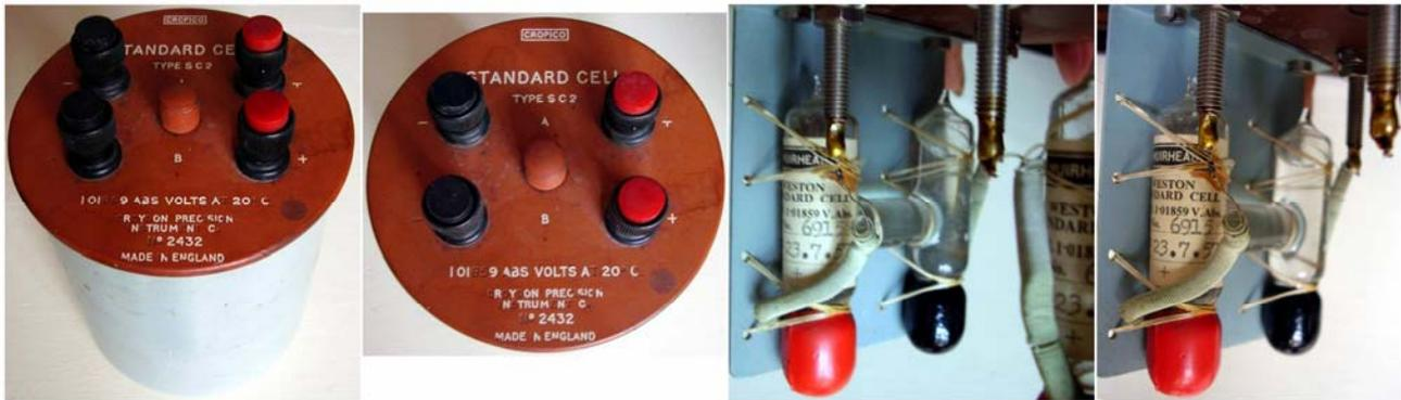
The Weston cell was first devised in 1893 and accepted as primary voltage standard since 1911. Still today it is in semi-clandestine use to check solid state voltage references. Due to environmental restrictions for its major components, mercury and cadmium, its use is very limited and secret today. Unfortunately, even the documentation and the same datasheets have been removed from the Web, probably fearing mercury contamination of the keyboards!
